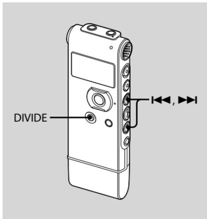
You can divide a message during playback, so that the message is divided into two parts and a new message number is added to the newer part of the divided message. By dividing a message, you can easily find the point from which you want to play back when you make a long recording such as at a meeting. You can divide a message until the total number of messages in the folder reaches 99.
