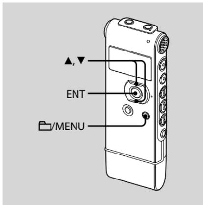
During FM reception or FM recording, you can switch between the sound from the speaker and the sound from the headphones using the menu. The FM radio output is set to “HEADPHONES” when you purchase the IC recorder.
