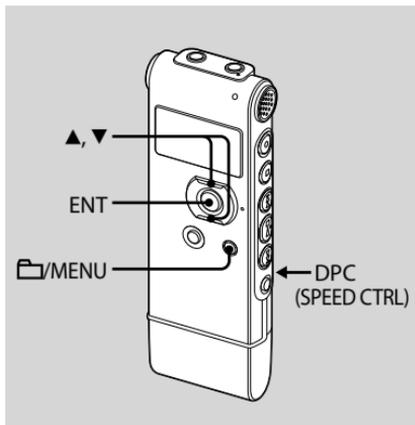
When you slide the DPC (Digital Pitch Control) (SPEED CTRL) switch to "ON," you can adjust the playback speed between +100% and -50%\* of normal speed in the menu.
