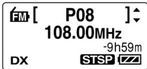
You can switch the display between preset number and frequency by pressing ENT.
