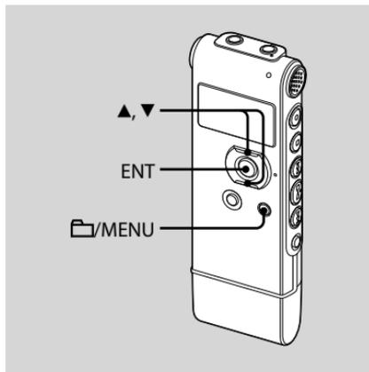
When you set the LCF (Low Cut Filter) function to "ON" in the stop or recording mode, you cut out a low frequency to reduce the roaring noise from wind, etc.; therefore you can record a message more clearly. The LCF function is set to "OFF" when you purchase the IC recorder.
